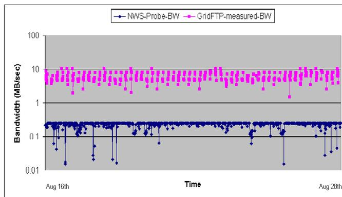
**Figure 1: LBL-ANL GridFTP (approximately 400 transfers at irregular intervals) end-to-end bandwidth and NWS (approximately 1,500 probes every five minutes) probe bandwidth for the two-week August’01 dataset.**
