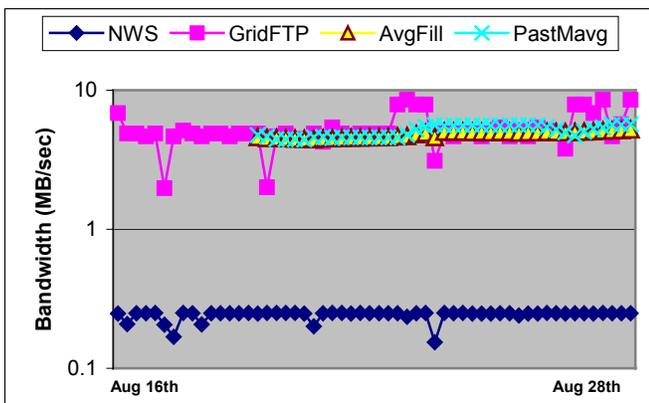
**Figure 6: NWS, measured GridFTP, and GridFTP predictions using linear regression with average filling and predictions using the moving average past predictor for 100 MB file transfers between LBL and ANL. Predictions include an initial training set of 15 values.**
