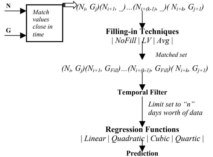
**Figure 3: Algorithm for deriving predictions from GridFTP (G) and NWS (N) data streams by using regression techniques.**
