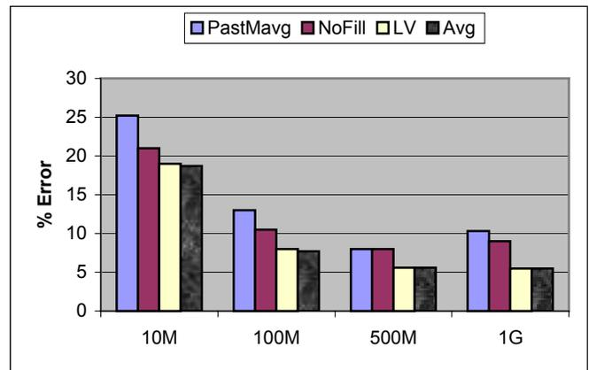
**Figure 8: Prediction accuracy using filling-in techniques for all file transfers between ISI and ANL.**
