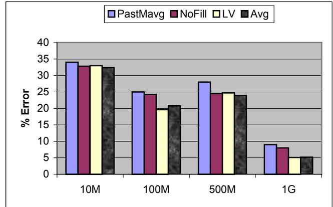
**Figure 7: Prediction accuracy using filling-in techniques for all file transfers between LBL and ANL.**
