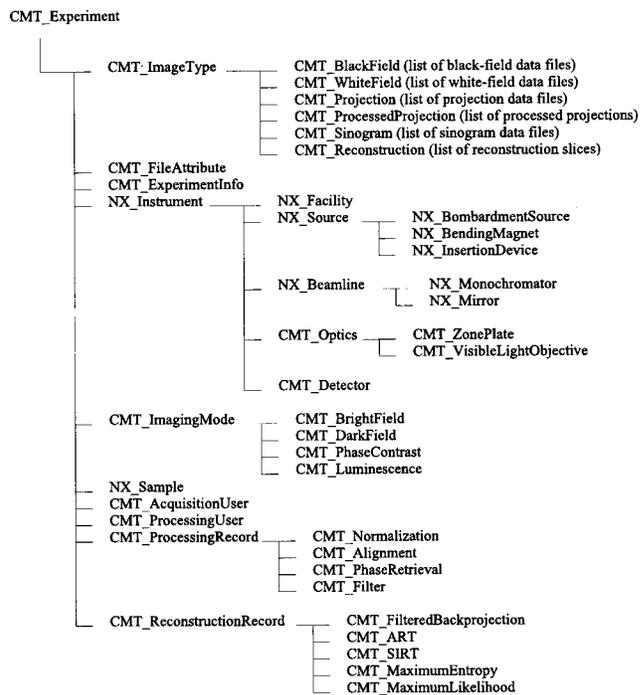
FIG. 4. Group structure of the tomographic data files. The CMT\_ImageType field contains an index of the data files containing black/white-field images, projections, sinograms, and the reconstructions. The information on the experimental conditions, users, sample, and computation parameters is stored in subsequent fields.
