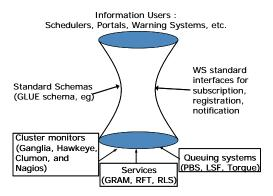
MDS4 builds on query, subscription, and notification protocols and interfaces defined by the WS Resource Framework (WSRF) and WS-Notification families for specifications and implemented by the GT4 Web Services Core.
